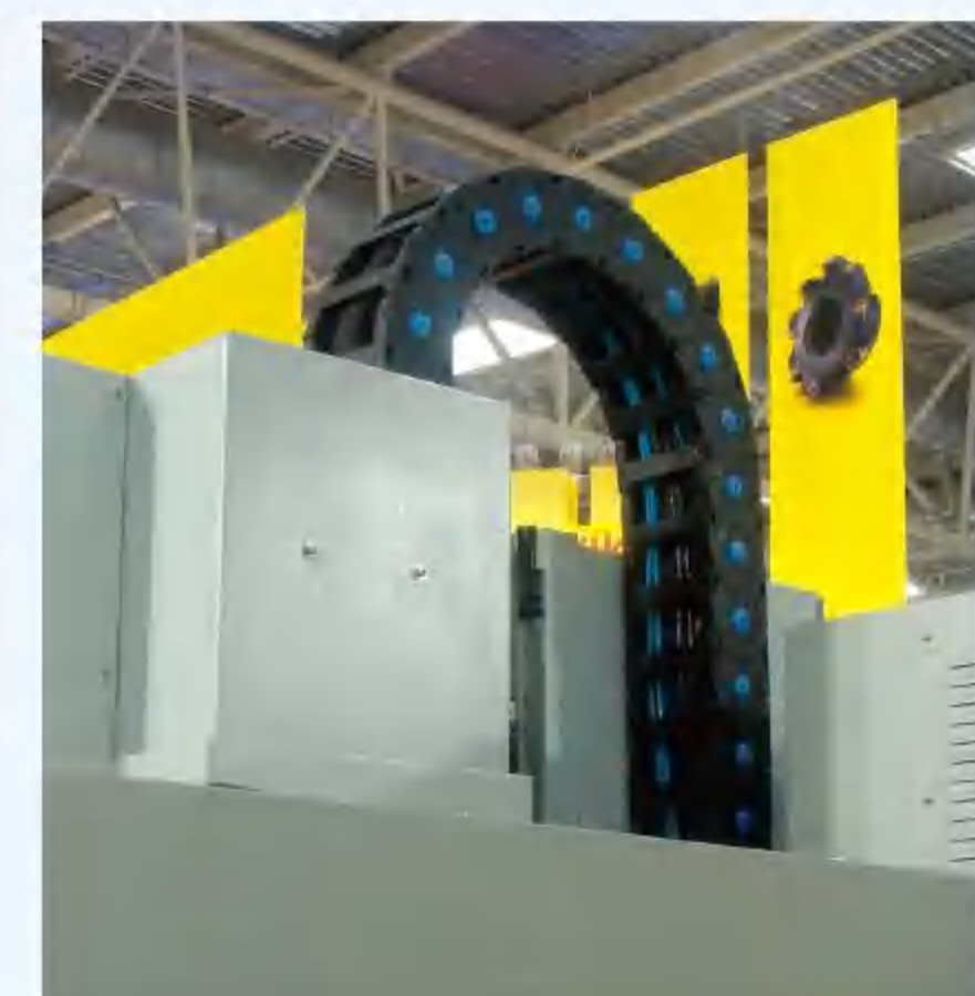
重叠实用的尼龙拖链应用在 石材机器上 Model Krius chains in nylon superimposed on a machine which works with marble.
