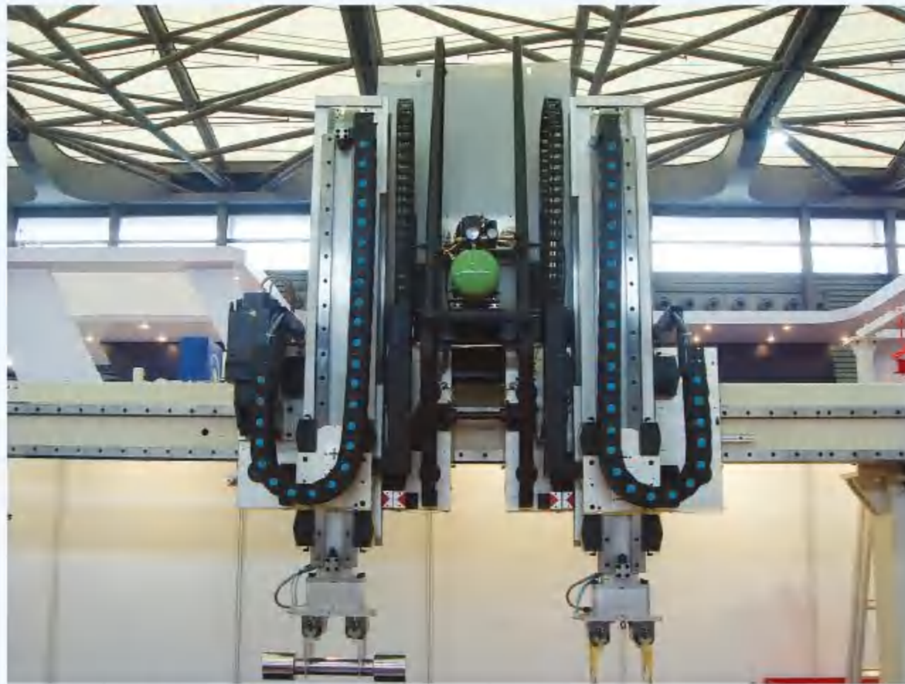
东方拖链用于机床上做下方是曲线的垂直运动 Dongfang vertical with curve below nylon chain on machine tool.
