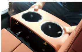
25.装回杯架底座拧回两颗螺丝
