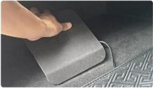
8.将多余电源线放入电池盒中并盖回上盖
