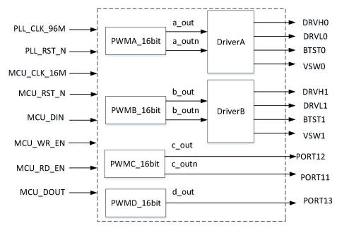
PWM A&B with the MOS deivers can driver a full bridge inverter, PWMC and external power stage to compose another full bridge driver to drive one coils, the single end PWMD is a controller for voltage regulating solution.
