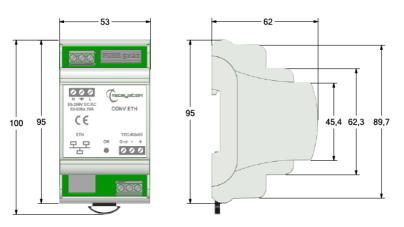
Secure the device on the DIN rail inside the panel.
