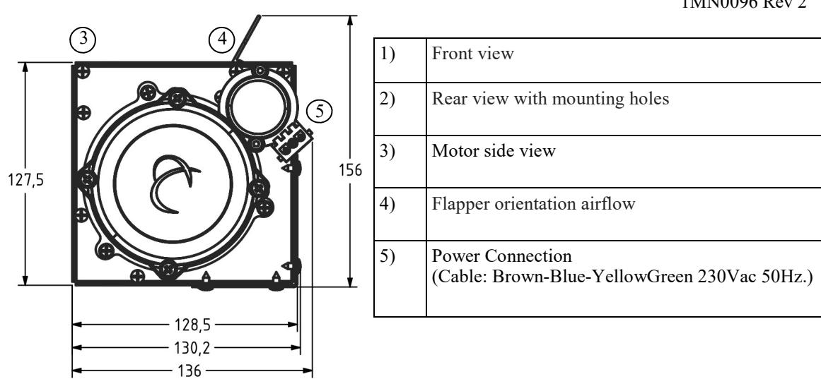
**DIMENSIONS (mm), MOUNTING HOLES AND CONNECTIONS TG500**
