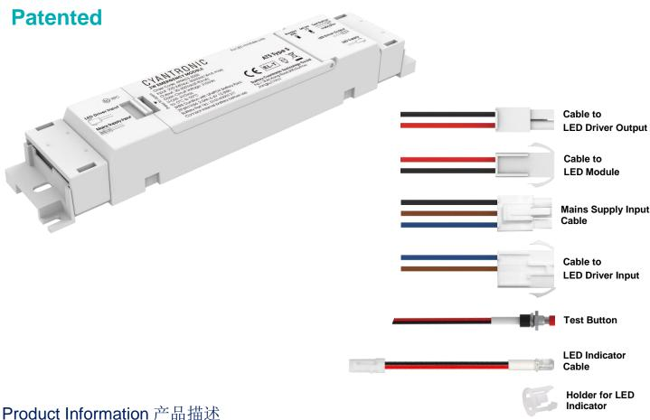
This emergency module can be used built-in for the LED linear luminaires with integrated LEDs. It is designed for installing within the fitting to provide a battery back-up supply in the event of a power cut. The emergency module requires a permanent live un-switched supply to maintain the battery charge. In the event of a power cut the battery will supply the luminaire at a reduced output.
