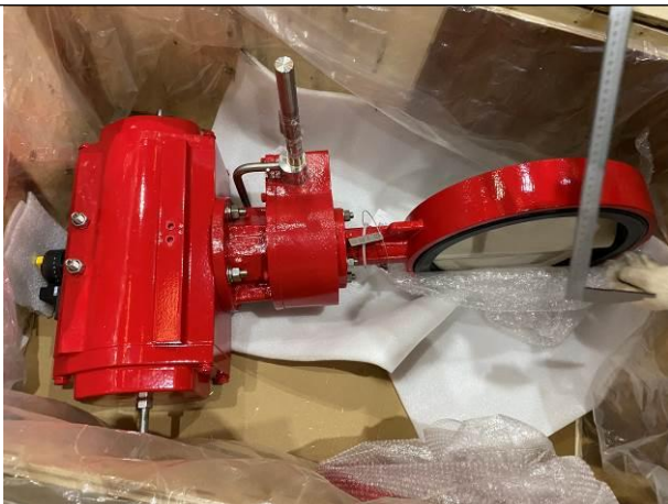
Visual inspection for butterfly valves
