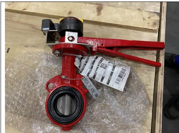
Visual inspection for butterfly valves
