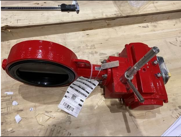
Visual inspection for butterfly valves
