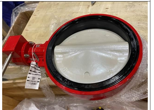
Visual inspection for butterfly valves
