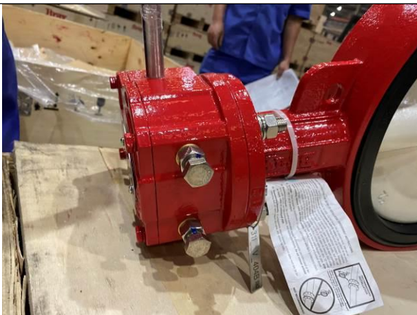
Visual inspection for butterfly valves
