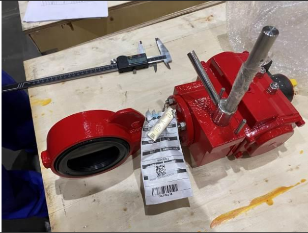
Visual inspection for butterfly valves
