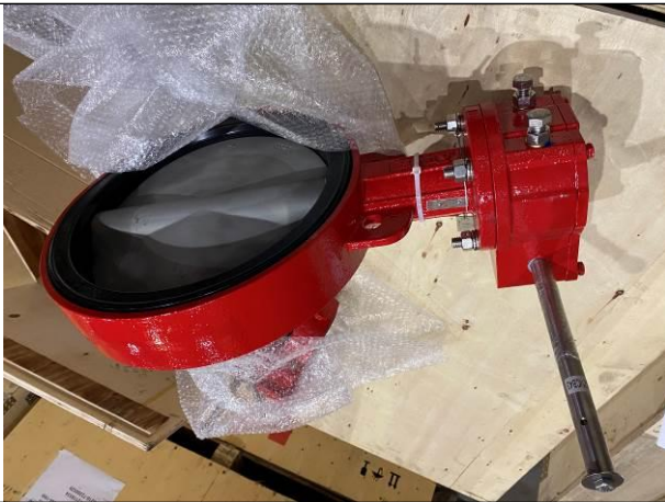
Visual inspection for butterfly valves
