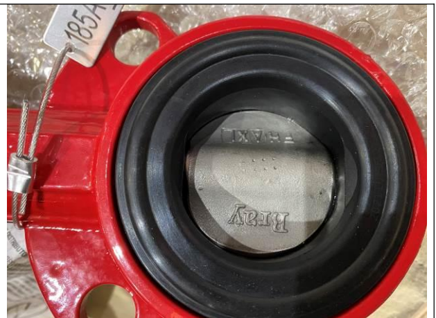
Visual inspection for butterfly valves
