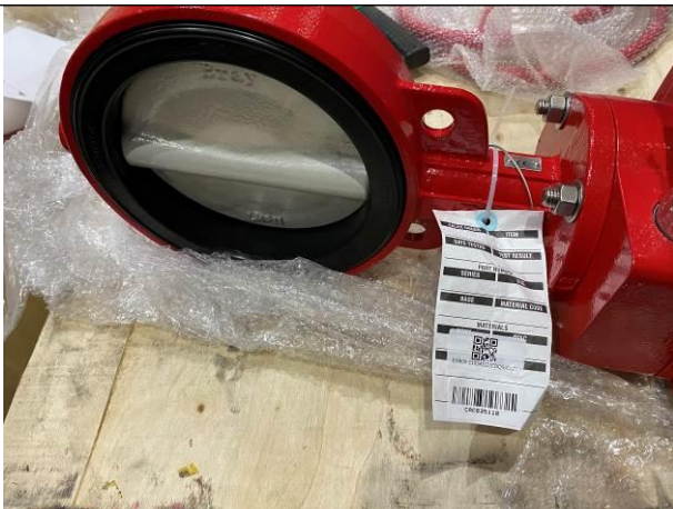
Visual inspection for butterfly valves
