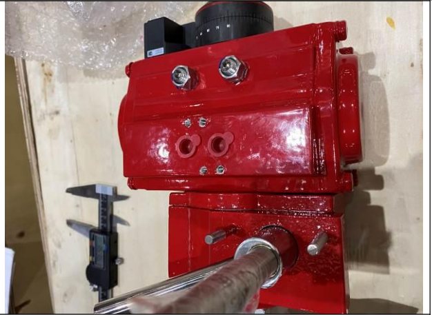
Visual inspection for butterfly valves
