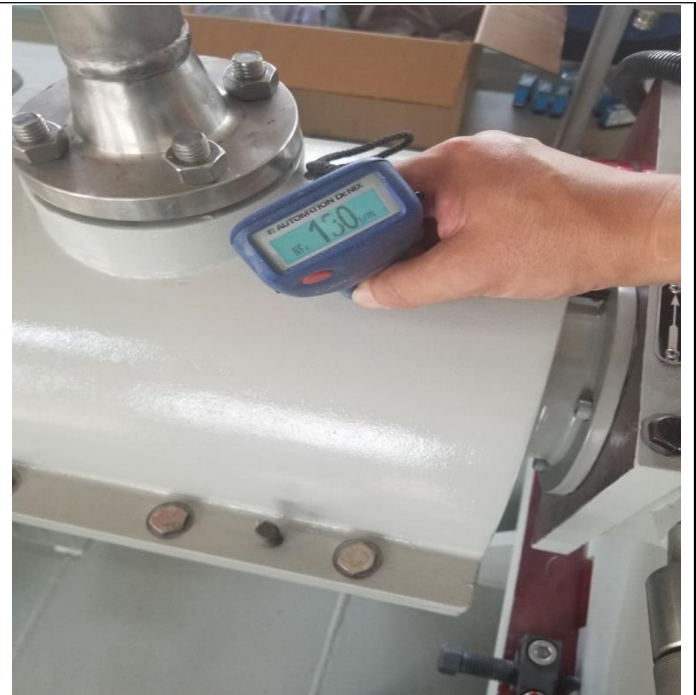
20. The thickness of the paint film on coupling cover is not thick enough and needs to be repainted(product no ***)
