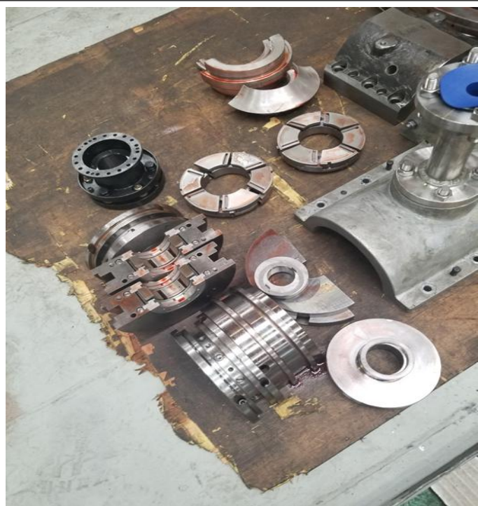
37. Rust proof inspection of bearing box and bearing surface(product no ***/***)
