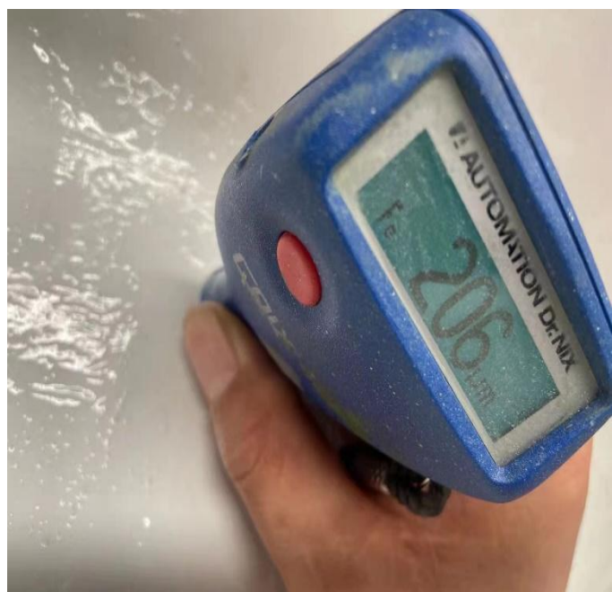
35. Film thickness measurement of *** / *** diaphragm
