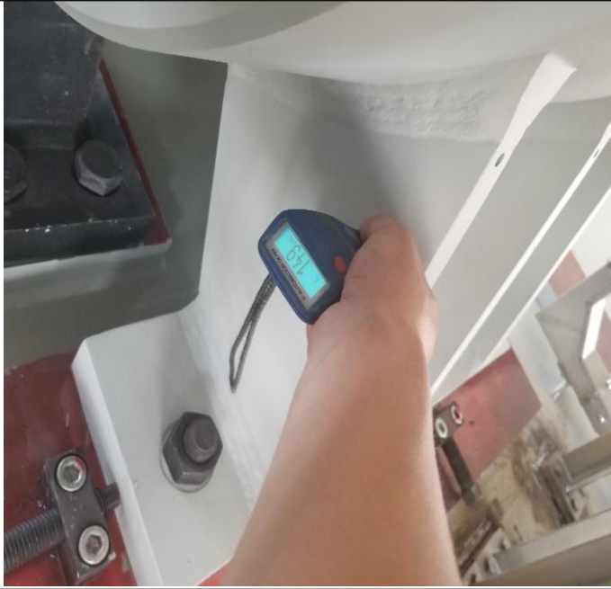
27. Inspection of paint thickness of compressor buttress(product no ***)
