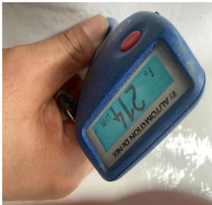
36. Film thickness measurement of *** / *** diaphragm
