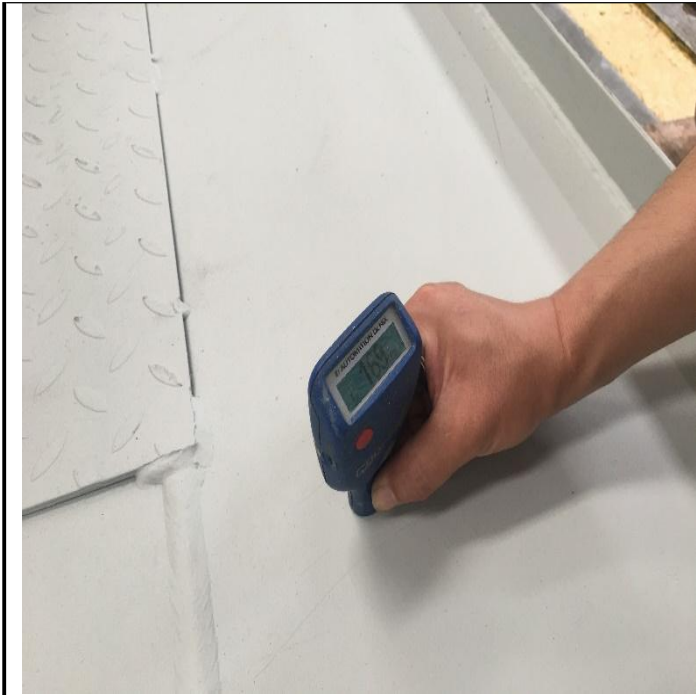
19. Inspection of paint thickness of base plate(product no ***)
