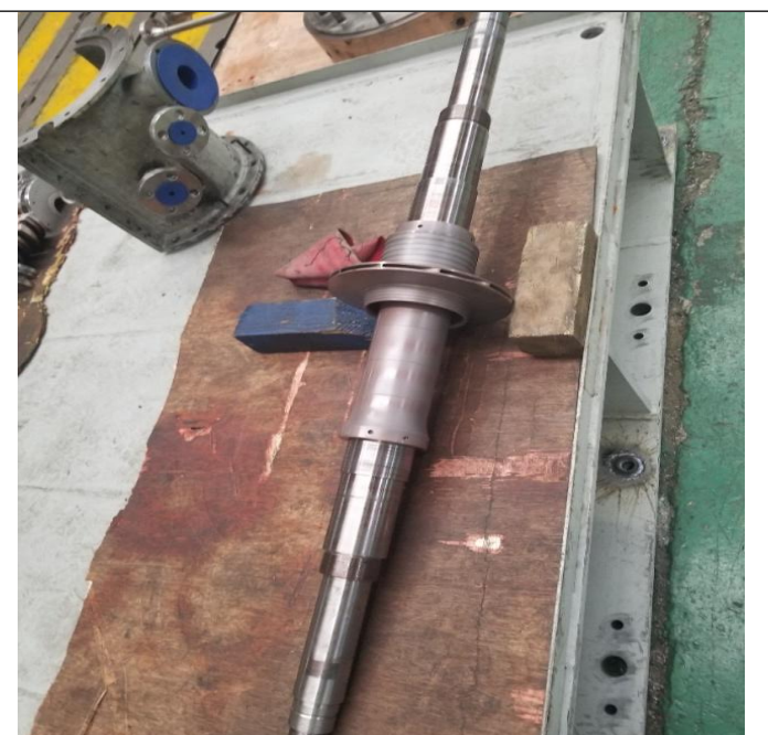
42. Rust proof inspection of rotor surface(product no ***/***)
