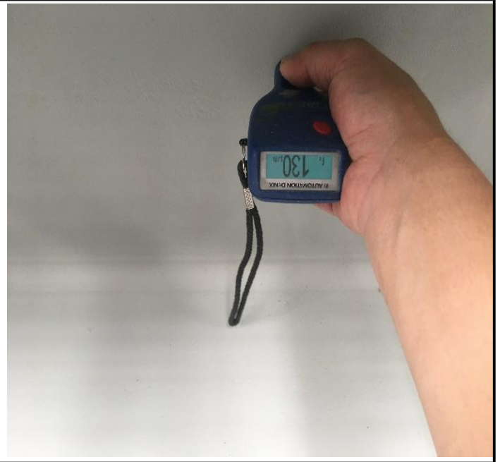
28. Inspection of paint thickness of base plate(product no ***)
