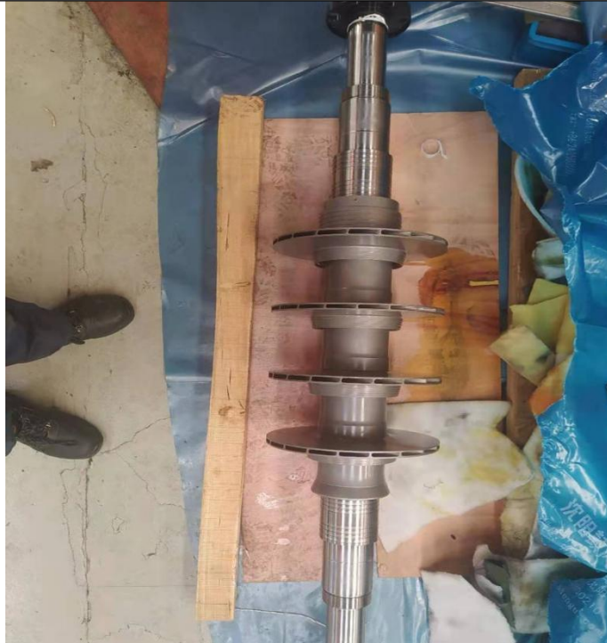
38. Anti rust inspection of rotor surface(product no ***/***)
