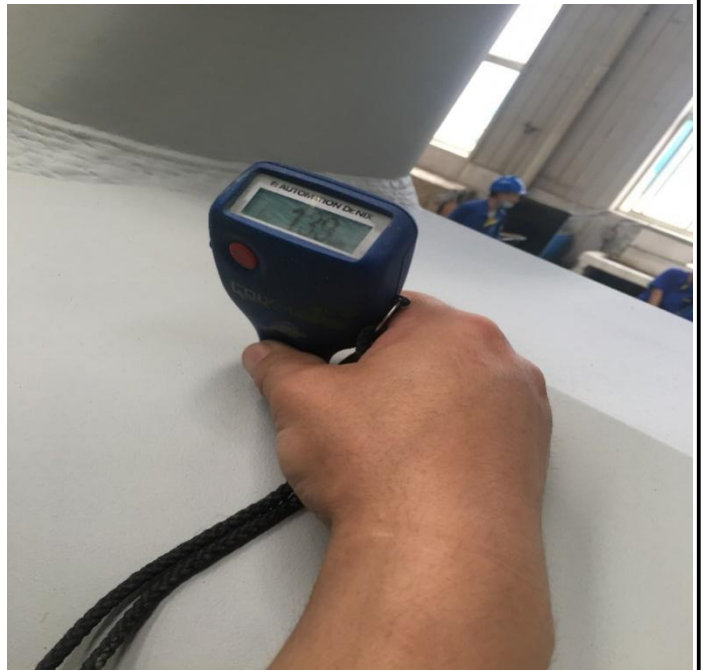
18. Inspection of paint thickness of compressor casing (product no ***)
