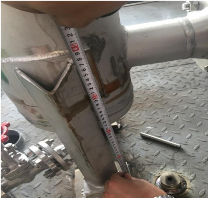
15. Height measurement of oil filter feet(product no ***)
