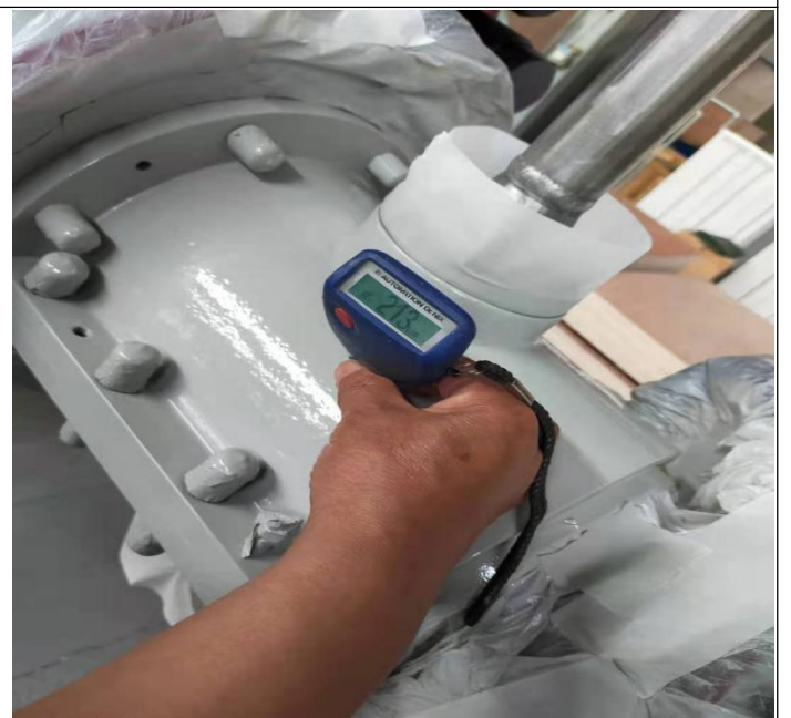
50. Film thickness measurement of *** coupling cover after repainting
