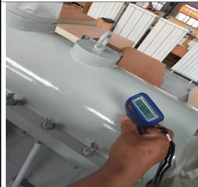
49. Film thickness measurement of *** coupling cover after repainting
