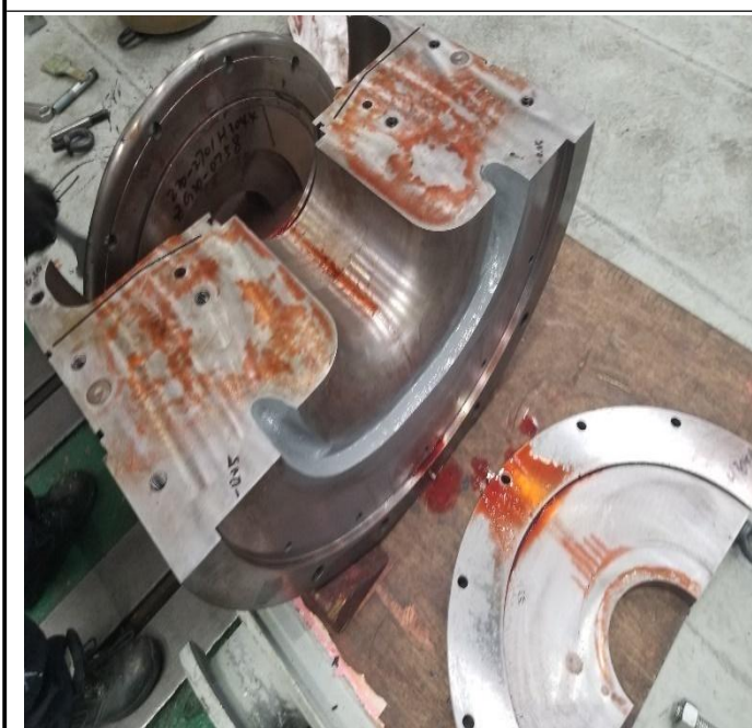
41. Rust proof inspection of stator surface(product no ***/***)
