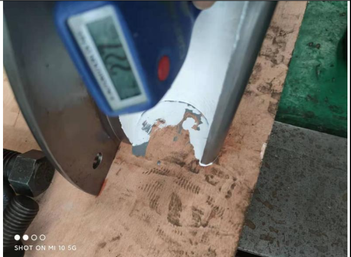
46. Film thickness measurement of *** / ***diaphragm
