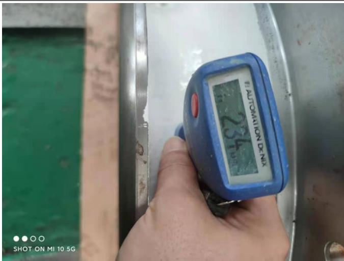
45. Film thickness measurement of *** / *** diaphragm
