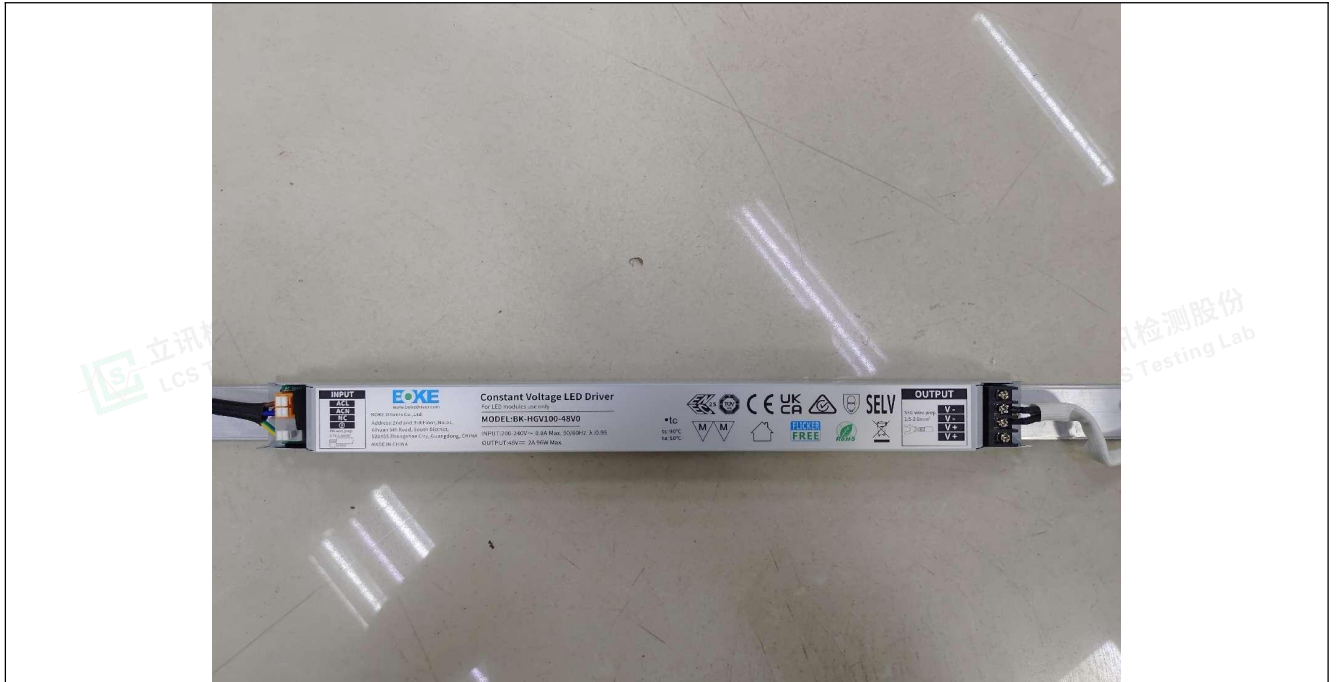
Photo 11 LED driver: BK-HGV100-48V0
