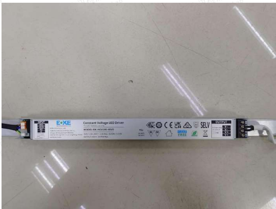
Photo.10 LED driver: BK-HGV100-48V0
