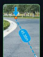
AR visual stakeout functionality provides real-time navigation quidance within the users' field of view. helping users quickly and accurately locate target positions for AR visual stakeout operations.
