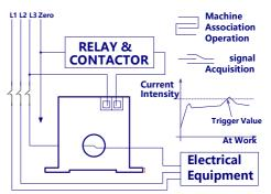
Switch contacts can pass AC DC current, connect inductive, capacitive and resistive loads, and can also be used as PLC signal collection.
